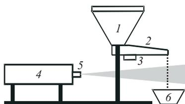
Fig. 1. A stand for pre-sowing laser treatment of seeds: 1 – charging hopper with metering device, 2 – chute, 3 – vibrator, 4 – laser, 5 – microscope lens, 6 – seed dish
